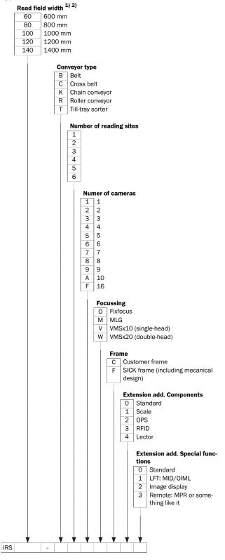
$<sup>^{1)}</sup>$  Assignment read field width: the tolerance is max. 50mm, e. g. at 650 mm read field width will be still a 060, 651 mm would already be a 080 system.
